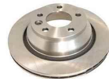
KP-VW-01180 BRAKE DISC 7L6615601G 7L6615601E TOUAREG MULTIVAN TRANSPORTER Diameter [mm]:314 Thickness [mm]:22 Minimum thickness [mm]:20
