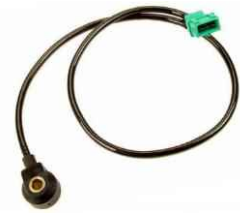
KP-VW-13080 Knock Sensor 0261231038 AUDI S4 ,V8 ,A4 ,A8
