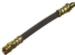
KP-VW-01233 BRAKE HOSE 893611775A PASSAT ,GOLF GL
