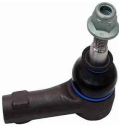
KP-VW-04053 TIE ROD END 7L0 422 818 B L=89 mm T1=M14X 1.5 T2=M16X 1.5 TOUAREG
