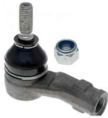
KP-VW-04038 TIE ROD END 191 419 811 L=75 mm T1=M12X 1.5 T2=M14 X 1.5 GOLF II GOLF III PASSAT
