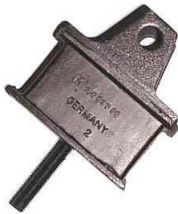
KP-VW-05078 Engine Mounting 070199231 VANAGON
