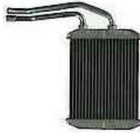
KP-VW-14145 HEATER CORE 377819030B
