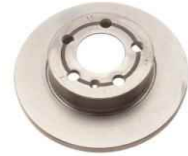
KP-VW-01200 BRAKE DISC 1J0615601D GOLF BORA Diameter [mm]:239 Thickness [mm]:9 Minimum thickness [mm]:8 Height [mm]:33,5
