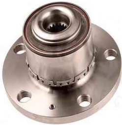
KP-VW-03001 WHEEL HUB 1J0598477 Inner diameter [mm]:63 Outer diameter 1 [mm]:30 Outer diameter 2 [mm]:65 Height [mm]:65 GOLF IV NEW BEETLE BORA
