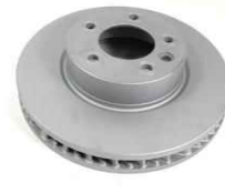
KP-VW-01195 BRAKE DISC 7L6615302D 7L6615302J TOUAREG Diameter [mm]:330 Thickness [mm]:32 Minimum thickness [mm]:30 Height [mm]:68,7
