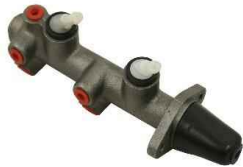
KP-VW-02009 BRAKE MASTER CYLINDER 113 611 015 113 611 016 149 611 015/2 Diameter [mm]:19,05 Thread Measurement 1:5xM10x1 KAEFER ILTIS
