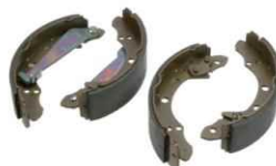
KP-VW-01055 BRAKE SHOE FSB273 443698525BX Diameter [mm]:200 Width [mm]:40 GOLF III
