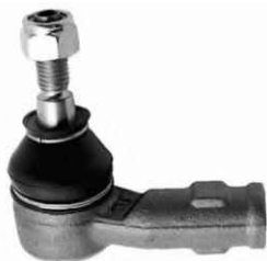
KP-VW-04042 TIE ROD END 1J0 422 811 L=75 mm T1=M12 X 1.5 T2=M14 X 1.5 GOLF IV
