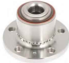
KP-VW-03002 WHEEL HUB 1K0498621 Inner diameter [mm]:29 Outer diameter 1 [mm]:27 Height [mm]:85 AUDIA3 GOLF V CADDY III Box
