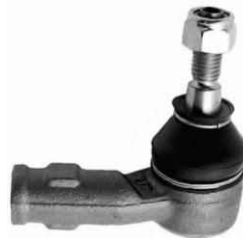
KP-VW-04043 TIE ROD END 1J0 422 812 L=75 mm T1=M12 X 1.5 T2=M14 X 1.5 GOLF IV
