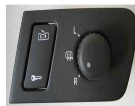
KP-VW-11116 MIRROR SWITCH 1T1 959 552 1T1 959 565 C 1T0 962 125 1T0 962 125 B Caddy, Touran (On Central Lock Switch)
