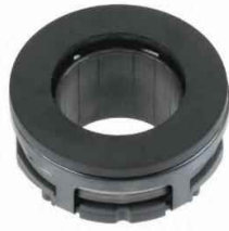
KP-VW-02065 CLUTCH RELEASE BEARING 01214165A 012141165B Outer diameter [mm]:42 Inner diameter [mm]:34 Height [mm]:23,9 Width [mm]:46,1 PASSAT PHAETON
