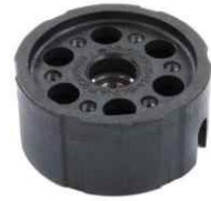
KP-VW-02068 CLUTCH RELEASE BEARING 02014165 020141165A Outer diameter [mm]:32,5 Height [mm]:18,9 JETTA GOLF POLO
