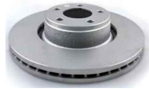
KP-VW-01204 BRAKE DISC 4F0615301D AUDI Diameter [mm]:314 Thickness [mm]:25 Minimum thickness [mm]:23 Height [mm]:59,5
