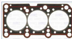
KP-VW-06051 CYLINDER HEAD GASKET Φ 83.5 mm AUDI A8 4.0 / 100 / A4 ETC
