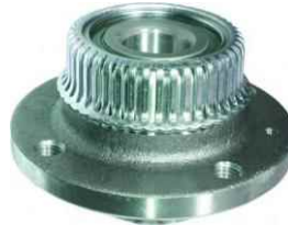
KP-VW-03011 WHEEL HUB 6X0598477 Inner diameter [mm]:28 Outer diameter [mm]:120 Height [mm]:64 POLO LUPO
