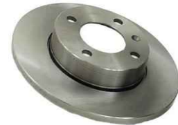
KP-VW-01176 BRAKE DISC 811615301 823615301 JETTA POLO GOLF PASSAT Diameter [mm]:239 Thickness [mm]:9,9 Minimum thickness [mm]:8 Height [mm]:38,5
