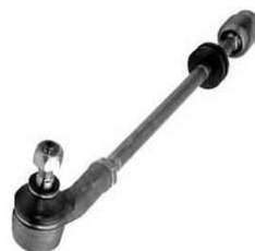
KP-VW-04247 Side Rod Assy 357419803 / 357419803A Passat (3A2, 35I) Passat Variant (3A5, 35I)
