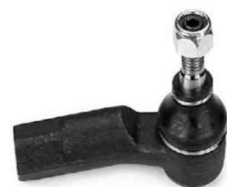
KP-VW-04048 TIE ROD END 1K0 423 811 C L=74 mm T1=M12X1.5 T2=M16X 1.5 PASSAT CADDY III TOURAN
