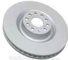
KP-VW-01202 BRAKE DISC 1K0615301M GOLF PASSAT Diameter [mm]:345 Thickness [mm]:30 Minimum thickness [mm]:27 Height [mm]:49,9
